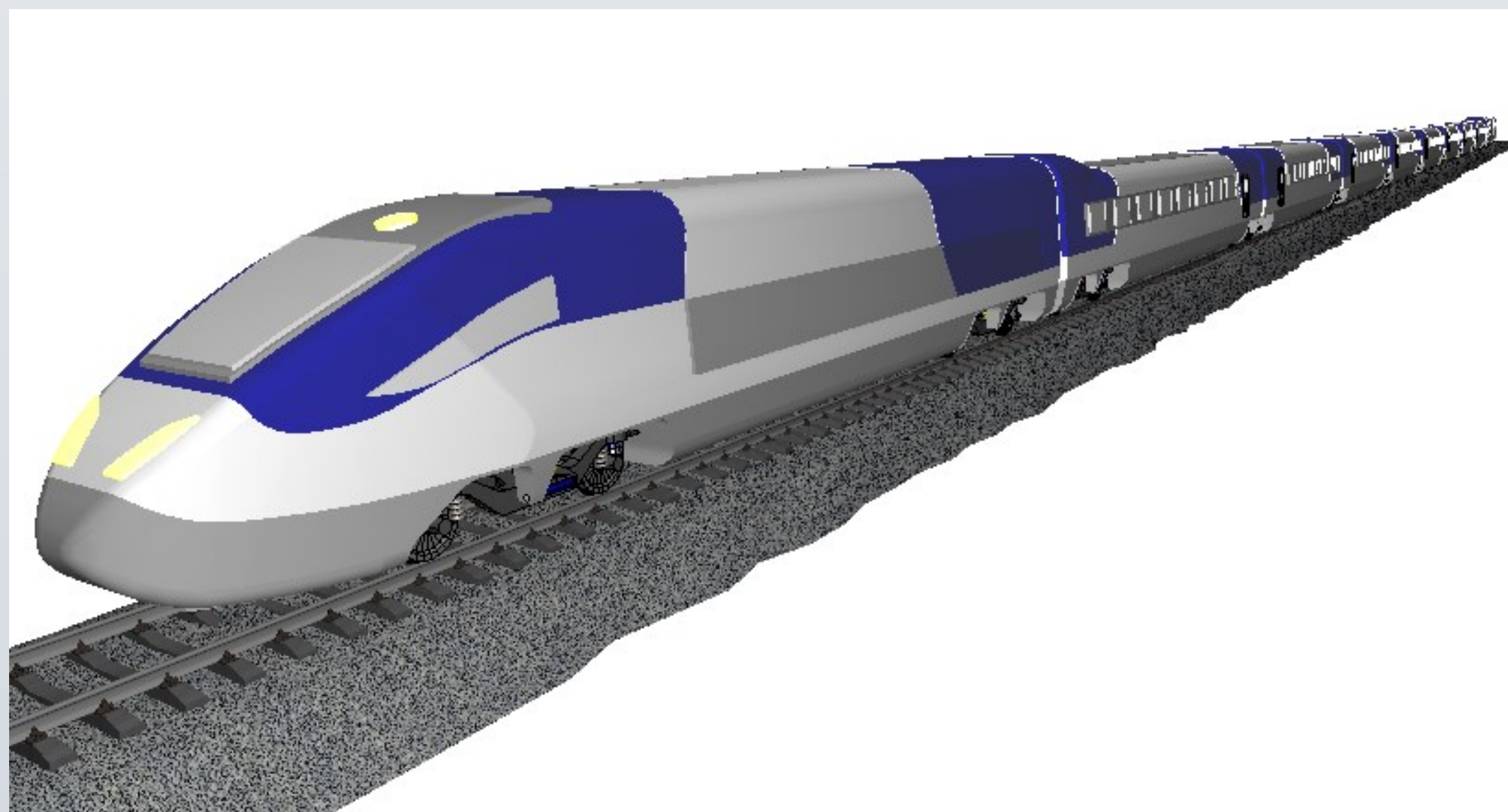
Figure 1. Multi-body model of high-speed train (TGV)
